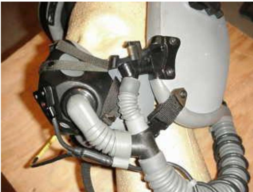
(Below: Two views of the TLSS assembly in 'Fighter,' or non-NBC configuration)
