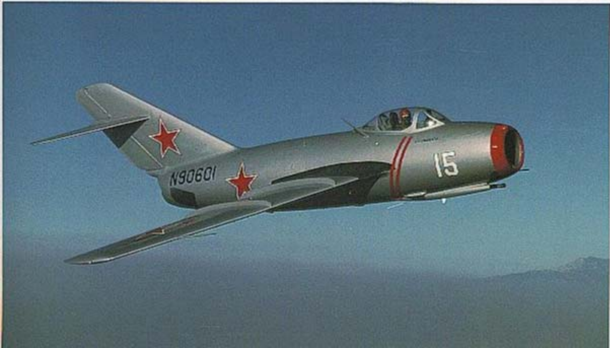
Russian MiG-15 (photographer unknown); note wing fences and cannons under nose.
