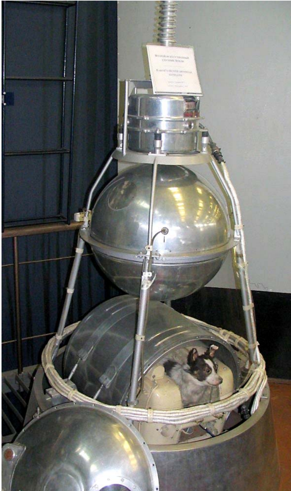
Model of the Sputnik-2 satellite, with external shroud removed; note viewing port.
