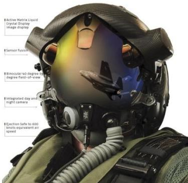
Figure 15: The new F-35 'smart' aircrew sensor helmet system
