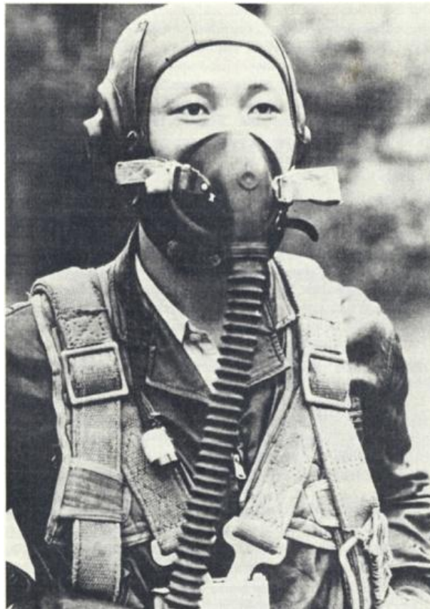
(Below: North Korean defector No Kum-Sok in his 1953 Chinese MiG-15 flight gear; shown is the Russian ShL-50 leather helmet and Russian KM-16A oxygen mask)
