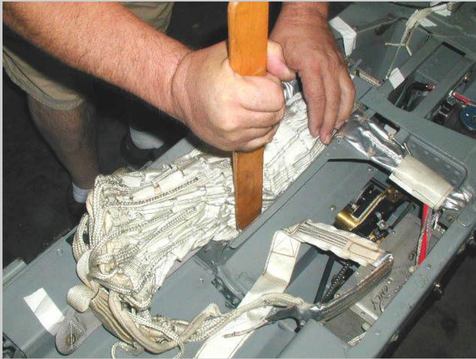
(Shown: tamping with fid is key to successful drogue assembly stowing process)
