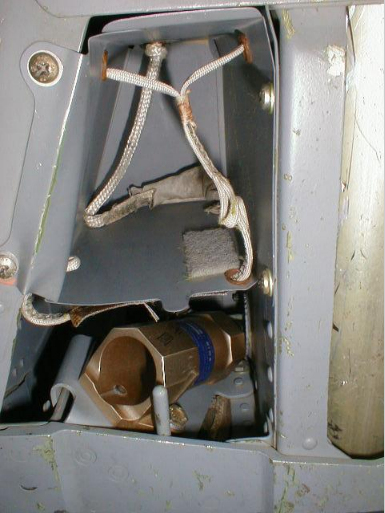
(Shown: upper extraction chute container detail on fired seat; drogue gun below)
